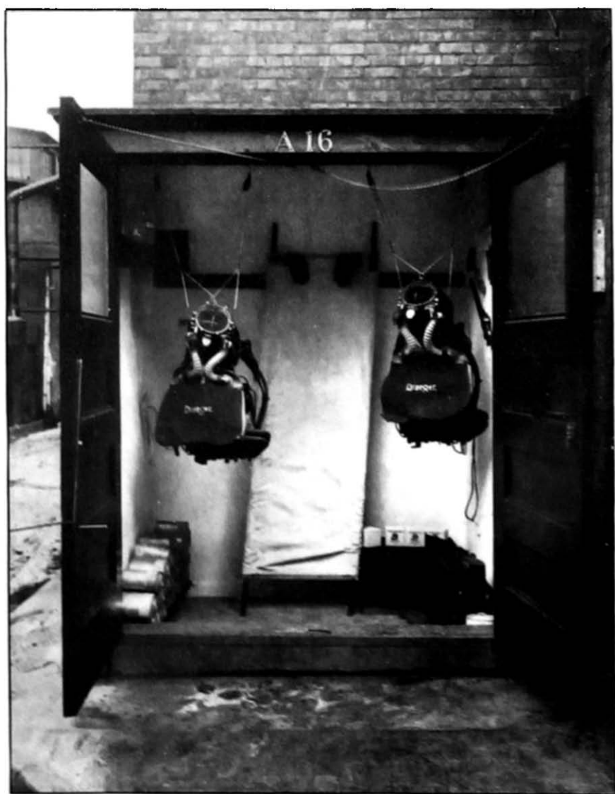
PLATE I.—EMERGENCY APPARATUS OF A CHEMICAL COMPANY. NOTE STRETCHER, HELMETS, GLOVES, BOOTS, TOOLS, ETC.
