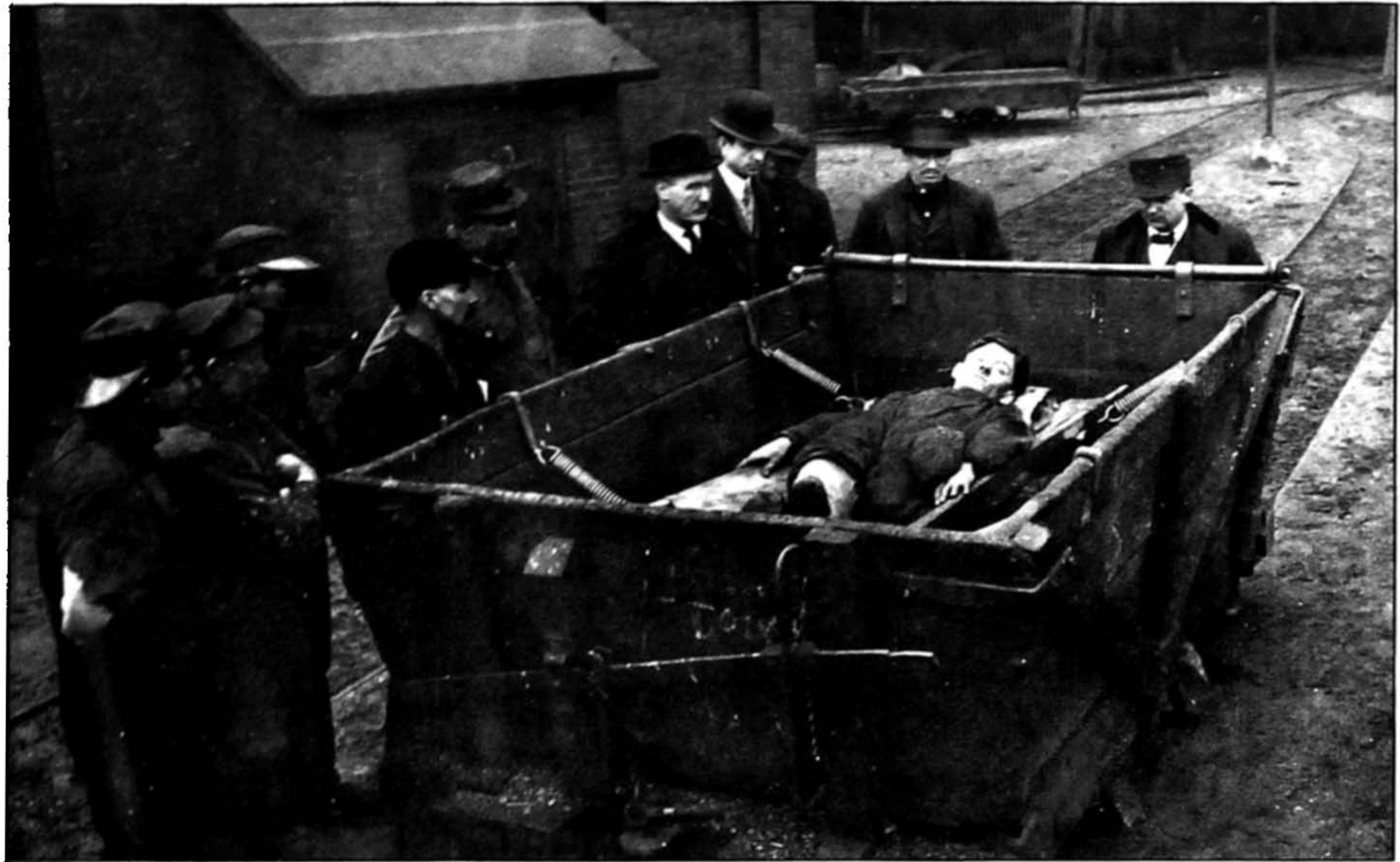
PLATE 8.—STRETCHER SUSPENDED IN MINE WAGON, WITH SPRINGS TO ABSORB ALL SHOCK AND JAR, TO TRAVEL FROM PLACE OF INJURY TO SURFACE.
