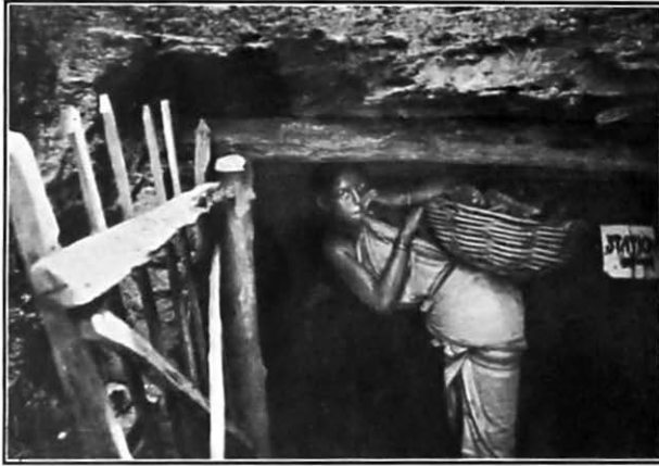
A WOMAN EMERGING FROM AN INCLINE. THE THICKNESS OF THE SEAM IS 4 FEET 6 INCHES, AND THE HEIGHT OF THE UNDERGROUND ROADS RARELY EXCEEDS THIS FIGURE. THE GRADIENT IS 1 IN 12. THE DISTANCE OVER WHICH THE COAL HAS TO BE CARRIED VARIES FROM 150 TO 250 FEET OF UNDERGROUND ROADWAY. THE WEIGHT OF COAL CARRIED IN THE BASKET IS ABOUT 60 LBS.
