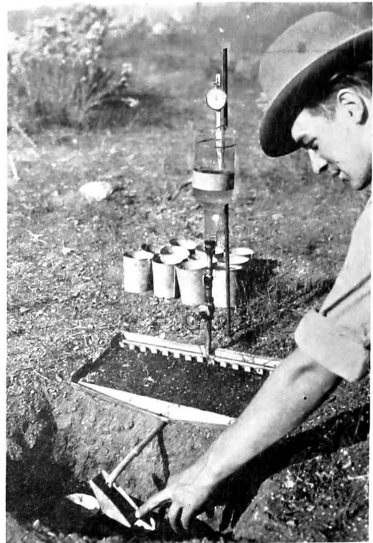
U. S. FOREST SERVICE FIGURE 22.—Apparatus used for simulating the conditions under which run-off from melting snow is absorbed by a soil in flowing over the soil surface. Developed and used by the Forest Service in the Boise National Forest.
