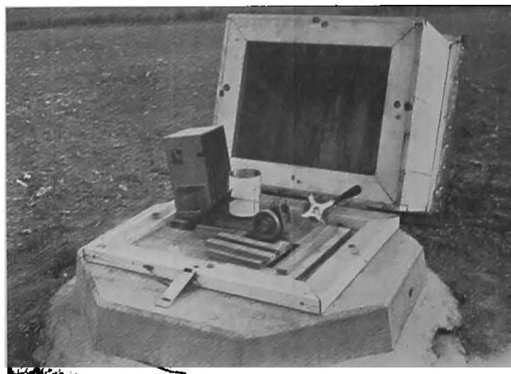
U. S. SOIL CONSERVATION SERVICE FIGURE 10.—A ground-water observation well showing the stage recording instrument installation, reference point, and well cover. Located at the North Appalachian Experiment Station, Coshocton, Ohio.
