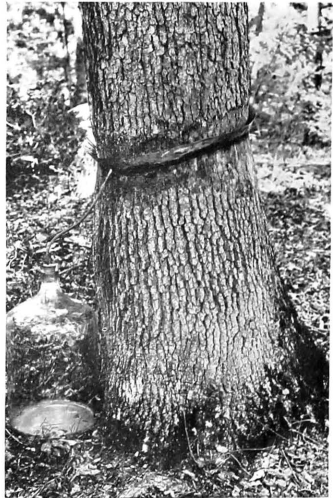
FIGURE 6.—A device for collecting crown intercepted precipitation, showing the collecting collar and container for determining the precipitation which would reach the ground by travel along the trunk.
