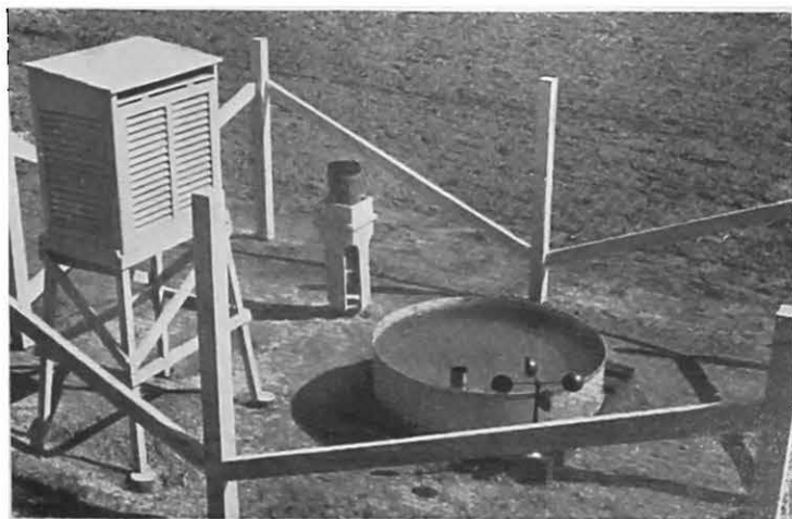
U. S. WEATHER BUREAU FIGURE 13.—A typical Weather Bureau first class station for the measurement of evaporation from water surfaces. From left to right the equipment includes an instrument shelter, an 8-inch standard rain gage, anemometer, and evaporation pan with hook gage well.
