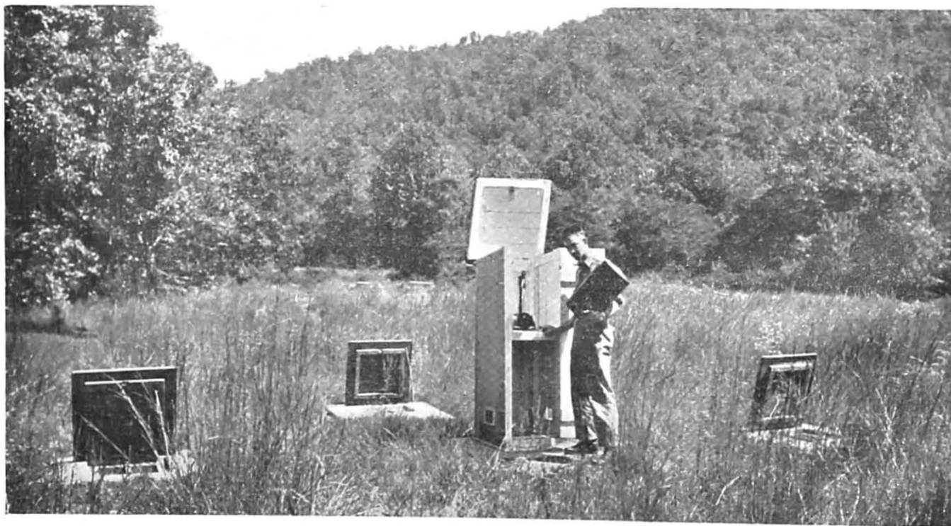
FIGURE 18.—Ground-water wells installed for the observation of ground-water levels and movements. Other groups of wells are located at intervals in and along the valley and the velocity of ground-water movement determined by electrical means. Coweeta Experimental Forest, N. C.
