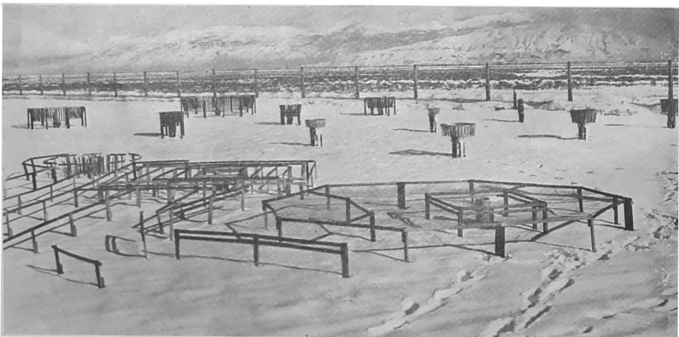
FIGURE 3.—Experimental shielded snow gages being investigated at Terminal, Utah. These consist of the standard 8-inch rain gage protected against air currents by movable and fixed shields of various designs. The studies include comparisons of the effect of varying the flexible shield shown in figure 2 both as to size and spacing.
