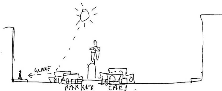
FIG 29: Glare, reflected from parked car tops obscures the central monument in city square
