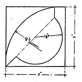
Complete marking out and cut to line with Hacksaw and Chisel.
