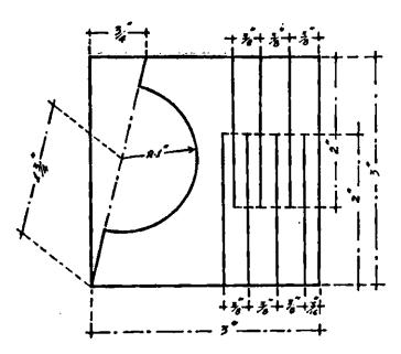
Complete marking out and cut to straight line with Hacksaw and curved line with Chisel.
