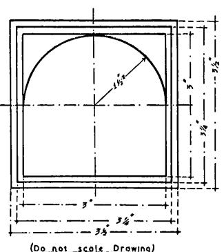
Part-1 Clean up workpiece scribe lines as Drawing and reduce to s'square by use of Chisel and Hammer.
