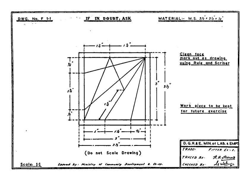
MATERIAL: M.S. 35 x 36 x 36 DWG. No. F 1-2 IF IN DOUBT, ASK Clean face mark out as drawing using Rule and Scriber Work piece to be kept for future exercise D.G.R.& E. Min. of LAB.&EMP TRADE - FITTER Ex. 2. (Do not Scale Drawing) CHICKED BY. L. D. Shorma Issued by: Ministry of Community Development & Co-op.
