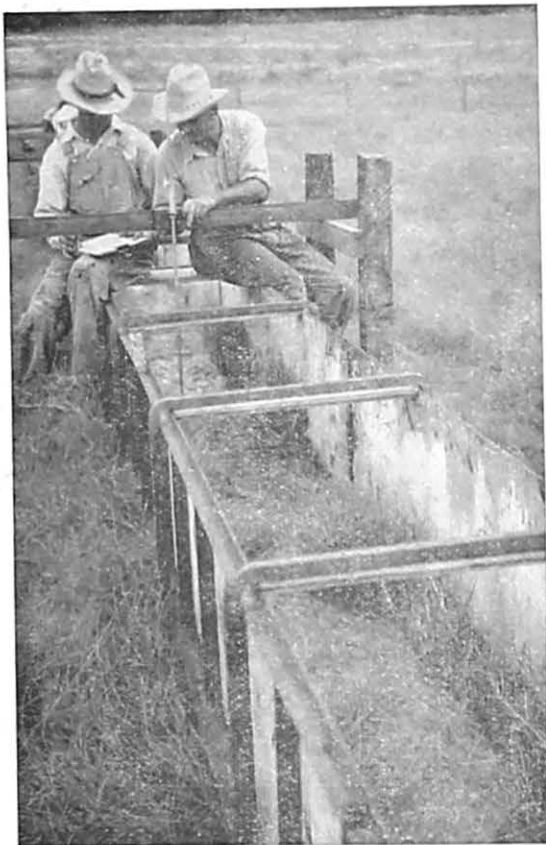
Fig. 6.—Equipment and procedure used in making bed and water surface observations. Bermuda grass Channel 7A, Experiment 1, with vegetation about 80 percent submerged.
