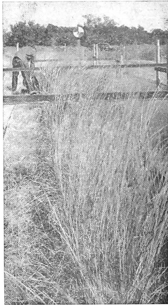
Fig. 11.—Native grass mixture in Channel 1D, Experiment 1. Little bluestem is the predominant grass, with growth as high as 48 inches.
