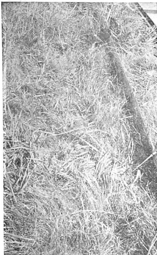
Fig. 9.—Buffalo grass lined Channel 10F before Experiment 1. The cover is 95 percent buffalo grass and 5 percent crabgrass.
