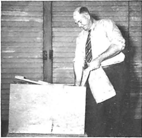
←STEP 3 Tightening baling cloth
