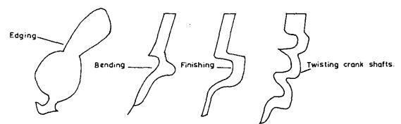
SHAFT FORGINGS : Stage of process I Edging II Bending III Finishing IV Twisting crank shafts
