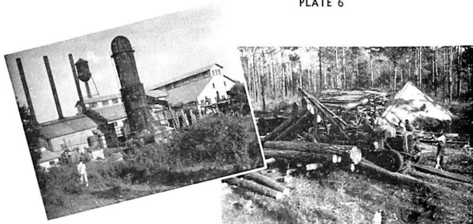
(Left) Trash Burner at Hardwood Sawmill. (Right) Logging Operations in South Carolina (Note saw dust pile and waste slabs in background).
