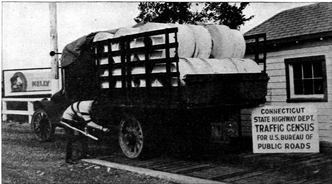
MEASURING THE WIDTH OF TRUCK TIRES TO DETERMINE THE WEIGHT PER INCH OF WIDTH
