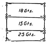
Rule 12.—If two numbers adjoin one another and the area of each is less than 20 gunthas, the marks must be erected according to Rule 11 above; but if a number whose area is less than 20 gunthas adjoins one whose area is less than 20 gunthas then the marks must be erected according to Ru'e 10 above.
