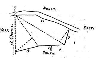
The length of the bases and perpendiculars shown by the interior dotted lines, and the calculation of the area of the field, are here inserted.
