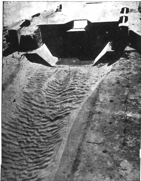
Photo 5179 : Photo showing final scour with 25 per cent retrogression in d/s water level; the design was the same as in photo 5173.
