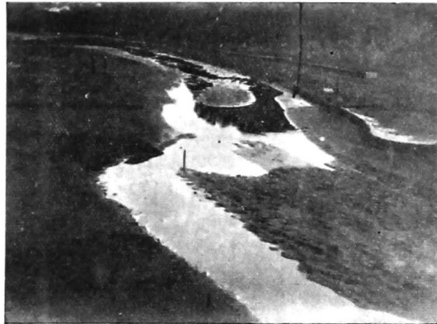
Photo 3055 : Photo looking downstream from left bank above groyne 4 showing the model channels as laid before beginning experiments 5 and 6, with pitched bank on right bank upstream of Pumping Station. This photo was taken at the beginning of experiment 6 in which the nose of groyne 5 was receded.
