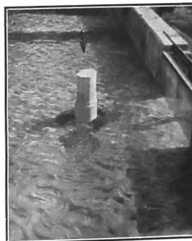
1085. Pier with loose stone protection after scour (looking upstream). Pier was fixed with axis at 15^\circ to direction of flow.
