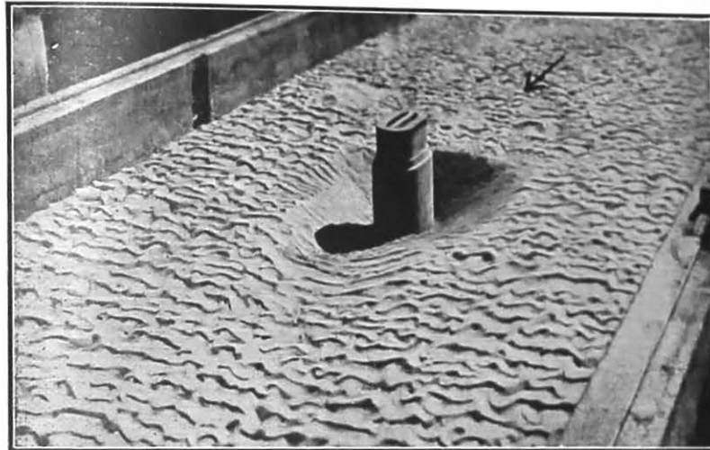
1410. Showing cup-shaped scour round pier with no stone protection (looking upstream).
