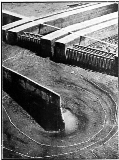
521. Showing a 'part' width model of the Sukkur Barrage showing deep scour at the vertical nose of the Divide wall.
