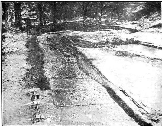
1580. Showing scour after 2 hours' ( \cong 9-5 hours) flow of Q \cong 12,500 cusecs in experiment 2 above.
