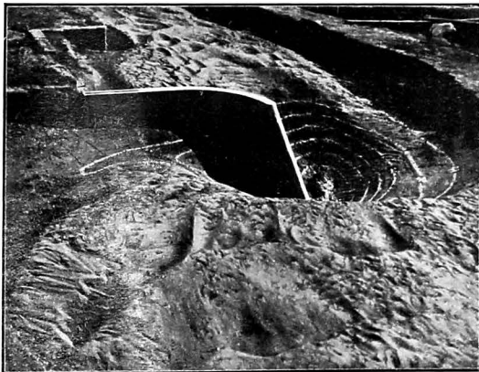
1670. Part-width model. Experiment 6. Burma type spur, showing very deep scour at nose. Looking downstream.
