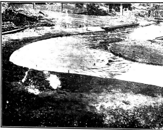
1517. Looking downstream. The spur in action: Discharge in model=6.28 cusecs ( \cong 32,500 cs., with 4 ft. depth over causeway).
