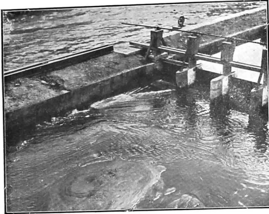
1256. A part-width model of Sukkur Barrage before downstream protection was added.
