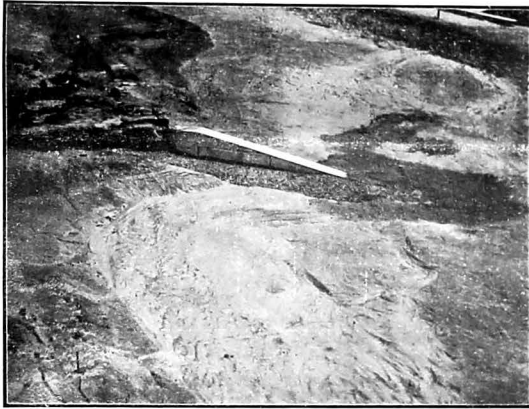
1669. Part-width, geometrically similar, model. Experiment 4. Sloping spur with mobile protection as laid before flood. Looking downstream.
