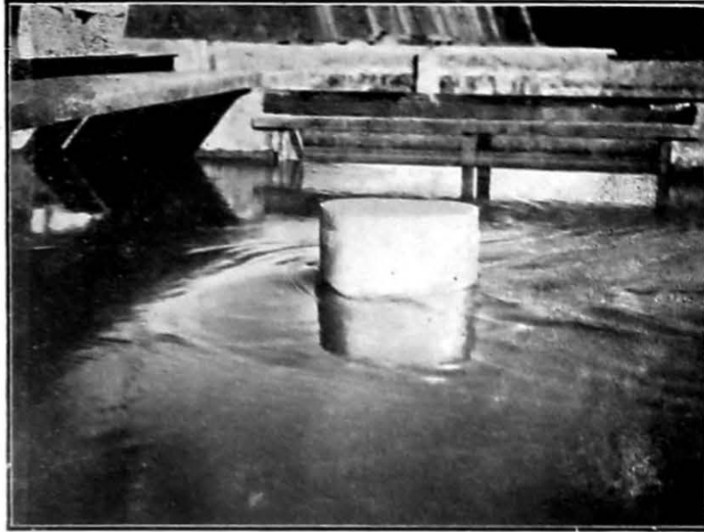
Photo 1012. Pier experiments showing water profile at pier.
