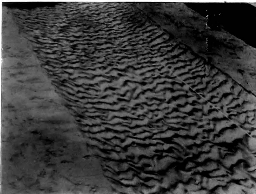
Photo 2289. Photo looking upstream in sand channel experiments, showing typical ripple formation in white V sand (unscreened), 0.24 mm., with Q = 1.5 cusecs without sand injection.
