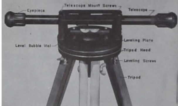
Figure 4. Gunscope type level showing parts.
