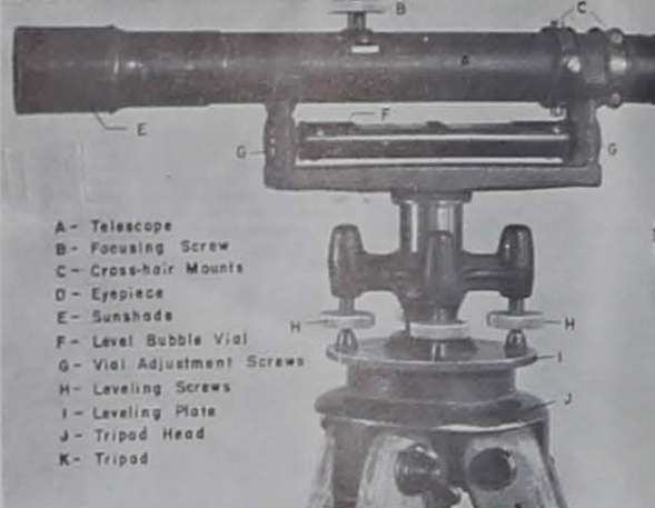
Figure 2. Utility type level showing parts.
