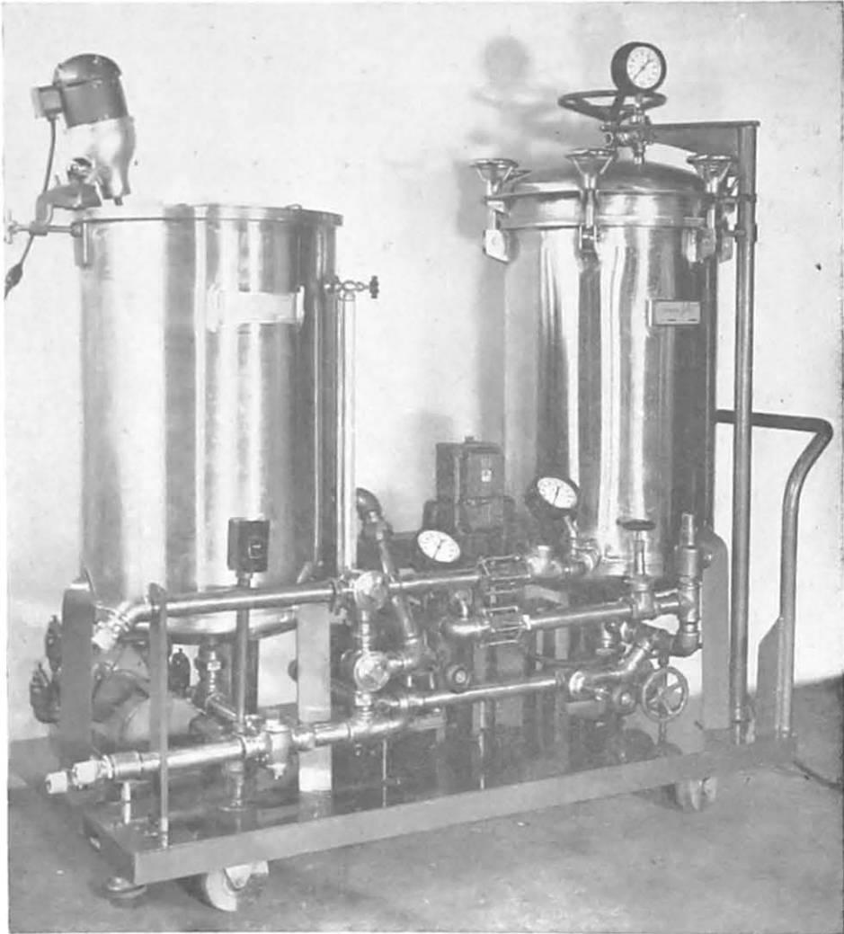
FIG. 18. Cylindrical Filter with Precoat Tank
