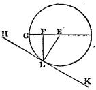
by the fulcrum LF. And the sphere, which is equal to the weight A, may be supposed to be collected at its center. If therefore B act at G, the weight A will be supported.
