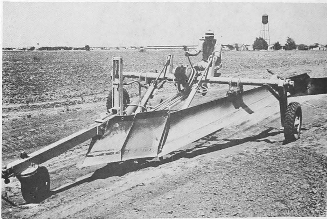
Photograph No. 56 Chattin Ditcher for excavating canals and laterals.
