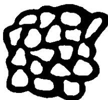
Figure 2. — Particles and water films in a saturated soil.
