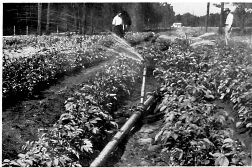
FIG. 6. Low-pressure revolving sprinklers operated by natural pressure from flowing artesian well. (Irrigating tobacco plants and early vegetables.)
