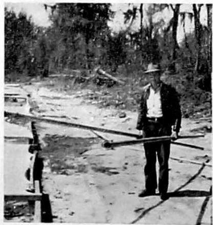
FIG. 10. Sprinkler-irrigation pipe is lightweight, is equipped with quick-acting couplers and is made in 20-foot lengths.
