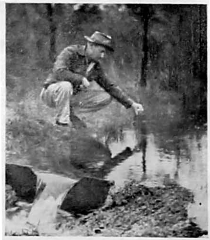
FIG. 8. Measuring flow of stream with portable 90° triangular-notch weir.
