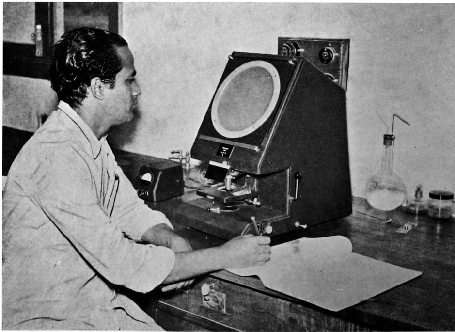
Measuring fibre cells with fibroscope at the Anatomy Section, Central Jute Agricultural Research Institute, Barrackpore
