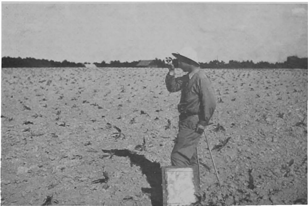
Figure 7.—Measuring the Slope of a Field with an Abney Level. This Surveyor is Making a Conservation Survey with an Aerial Photograph as a Base Map.
