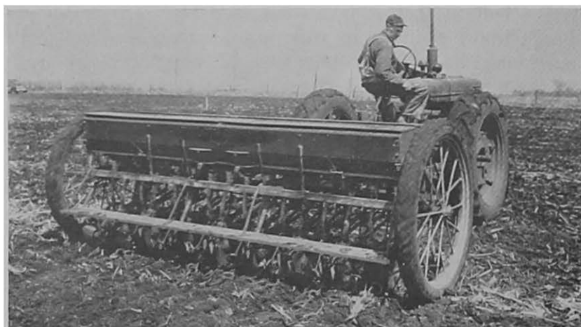
Fig. 11. The combination grain-fertilizer drill is the most effective method for applying fertilizer. This drill is being used on disked cornstalk land.
