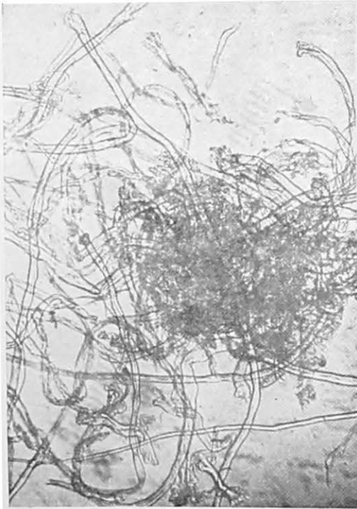
3. Damaged cotton fibre pieces in a nep \times 100
