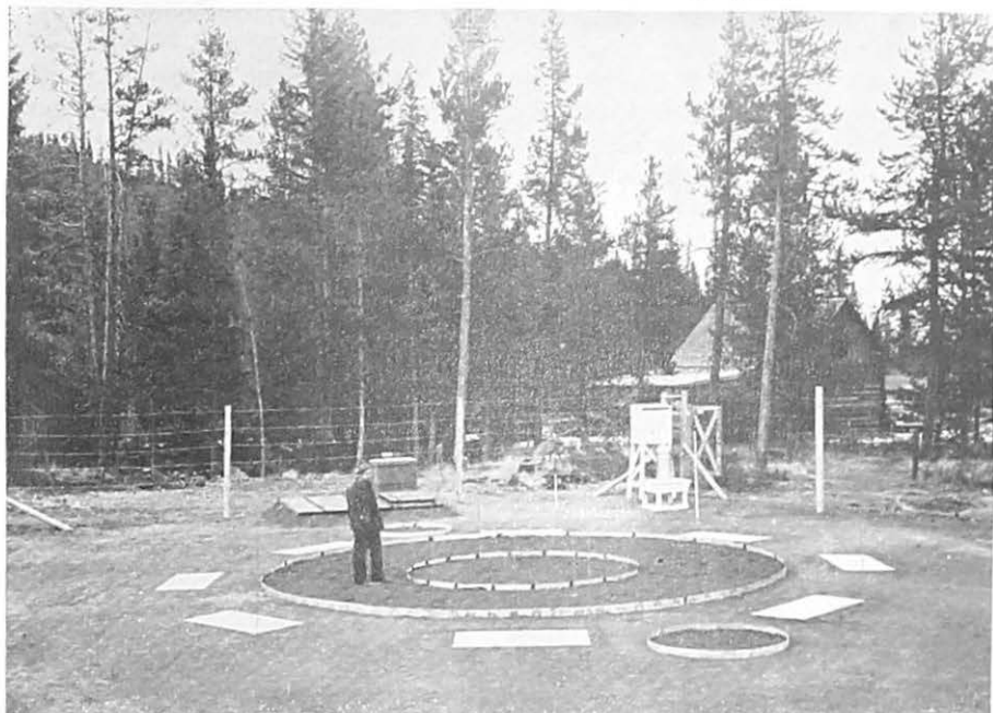
FIGURE 9.—Snow evaporation was measured with the aid of a pan 500 square feet in area. (Shielded snow gages were installed later.)
