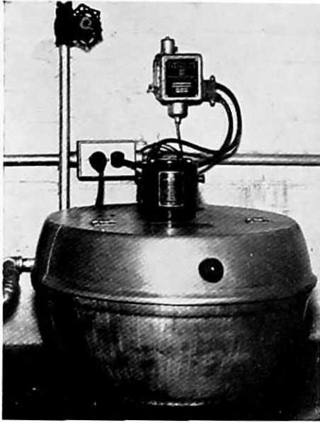
Electrically operated centrifuge, with thermostat, speed indicator, and thermometer. (Fig. 2)
