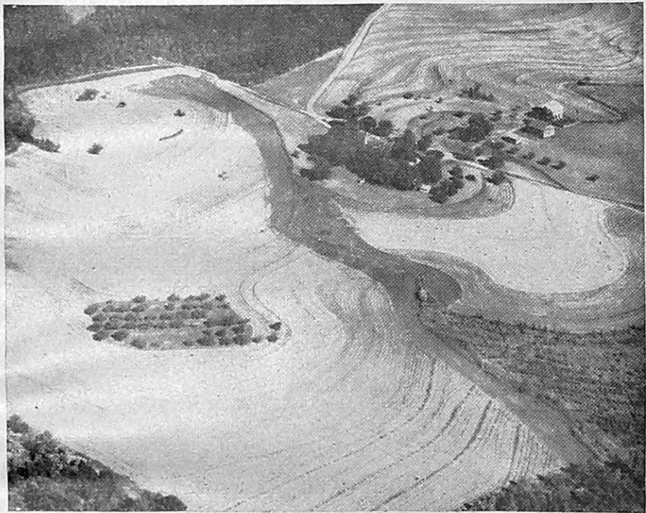
FIGURE 14.—A complete system of terraces discharging into a meadow outlet. This water-disposal system provides a complete foundation for conservation farming that will increase and maintain crop yields.
