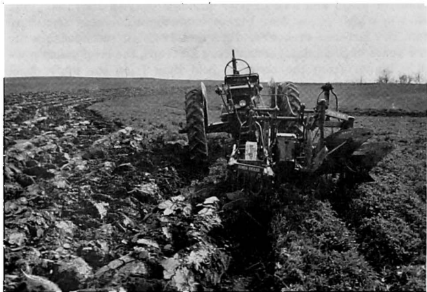
The two-way plow being used to plow terraces. No dead furrows or back furrows are left between terraces to concentrate water.
