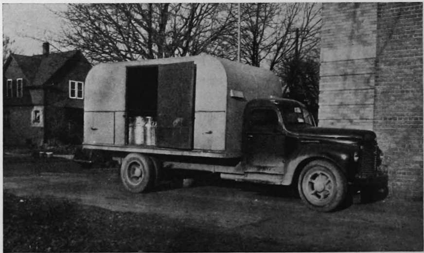
Figure 17. Insulated milk-hauling truck of the type shown here serves to protect milk while in transit
