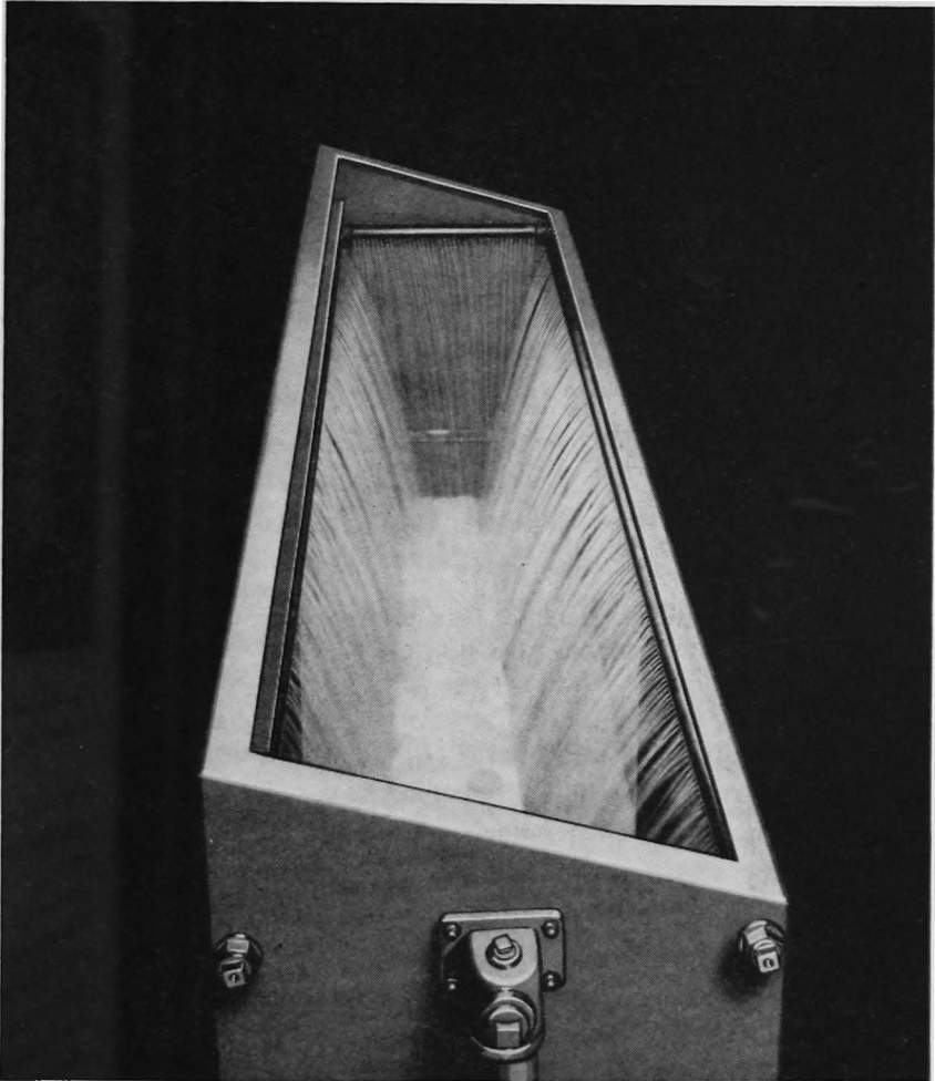
Figure 27. The spray method of heating milk in a vat. The inner lining has been removed to show how hot water is sprayed along sides and ends
