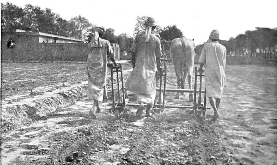
An improved triple Cotton Seed Drill with adjustable spacing. Set in this picture to 2 ft. 6 in.
