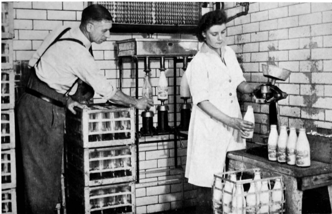
IN THE MILK ROOM AT POPLARS FARM, BRADFORD. MILK IS TRICKLING THROUGH THE COOLER, FILLING THE BOTTLES, WHICH ARE CAPPED BY MACHINE
