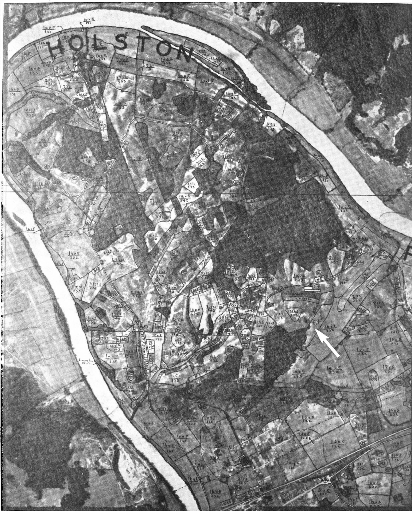
FIGURE 37.—Sample Section of Field Mosaic, Cross-Section Survey of the Upper Tennessee Valley
