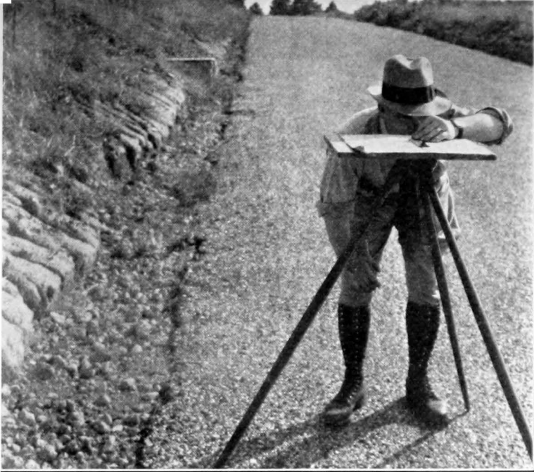
FIGURE 5.—Plane table assembled for use.
