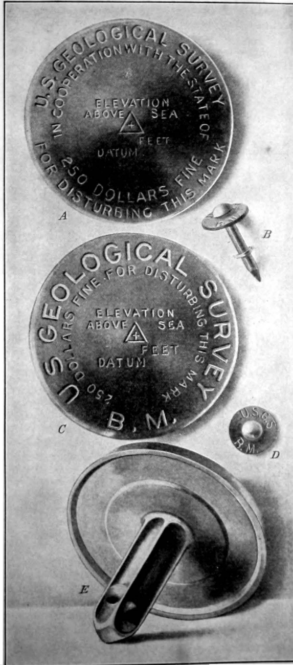
FIGURE 11.—Geological Survey station marks: A , Triangulation or transit traverse mark. (When used as the latter, the letters "TR" and the number of the station are stamped on the tablet.) C , Level benchmark. (Sometimes, at a later date, this benchmark may be made a transit traverse station, and it is then stamped with the letters "TR" and the number of the station. B and D , Copper temporary level benchmark.) (Courtesy United States Geological Survey)
