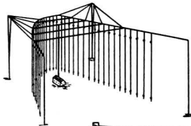
(d) MULTIPLE TUNED ANTENNA AND TRANSMITTER, 1919 NEW BRUNSWICK TRANSATLANTIC STATION
