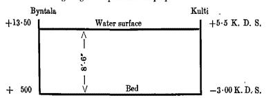
Subsequently in Annexure II to his note of 22nd December 1931 Dr. Dev showed the Dry Weather Flow channel with a water surface level of 15.00 K. D. S. at Byntala bed levels remaining as originally proposed. As Dr. Dev himself remarks the design is not good for
