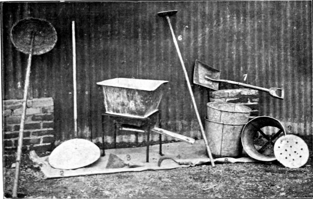
1 Shibe (for removing scum from the boiling pan). 2 Shibe (improved). 3 Hathia (wooden spatula). 4 Khurpa (scrapping hook). 5 Scum strainer. 6 Phavdi (wooden hoe). 7 Shovel. 8 Gul moulds. 9 Gul mould with false bottom.
