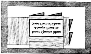
Fig. 84. Diagram showing proper positions of the inner quoins in the chase
