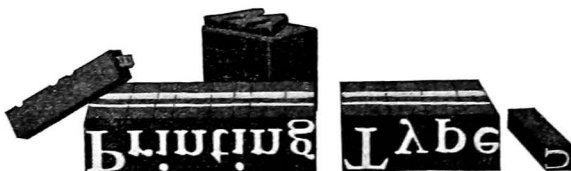
Fig. 13. Specimens of foundry type
