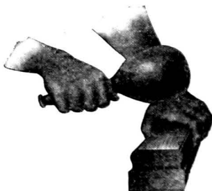
Fig. 55. Method of taking a stone proof
