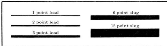
Fig. 26. Common thicknesses of leads and slugs
