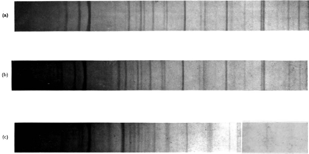
X-ray powder diagrams of (a) quartz, (b) a rock worker's lung residue, (c) an anthracite collier's lung residue ; (b) shows weak and (c) strong non-quartz lines.
