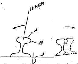
The outer rail had assumed the position shown in dotted line. Further on the inner rail was lying on its side and the outer rail also.
