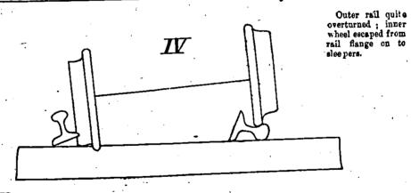
Between phase IV and phase V the inner wheel probably escaped to the position shown in phase V by bursting through the fish-plates.
