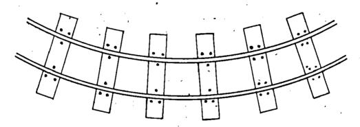
The rails appeared to have no inward inclination, and we formed the opinion that the original adzing had been done as in figure below:
