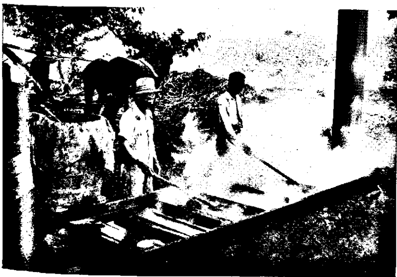
FIG. 112. Skimming the boiling juice in a sirup pan. Horse-drawn sweep-powered sorghum mill in background.
