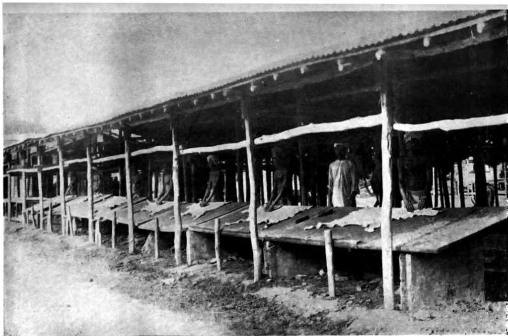
PLATE NO. 9—SETTING OUT HIDES WITH BRASS SLICKERS.
