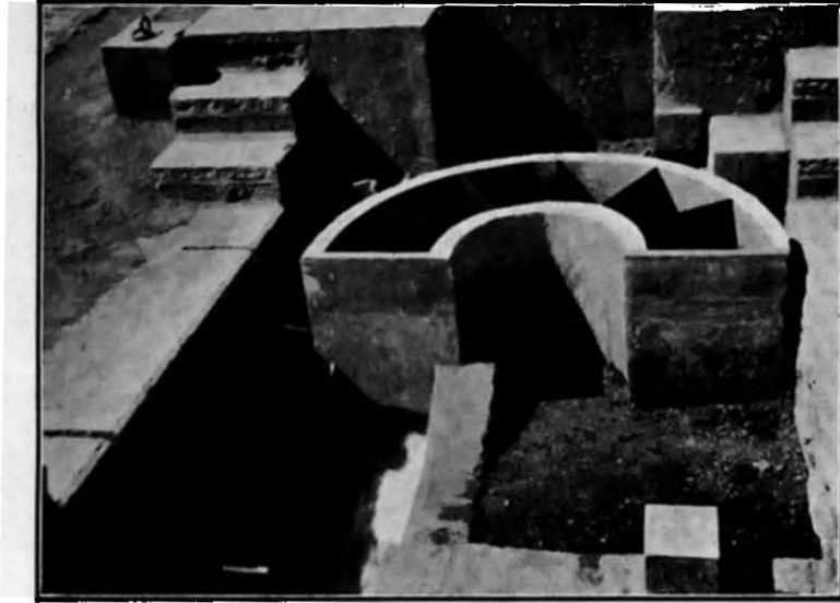
356.—3 cusecs Gibb module being tested in the Measuring Tank (Gibb's standard design).
