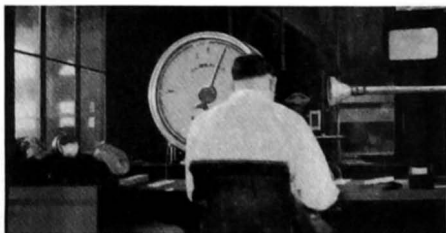
FIGURE 16.—LARGE DIAL SCALE USED AT SOME PUBLIC STOCKYARDS. Scales of this type enable patrons to see the weight registered, but they require careful servicing.
