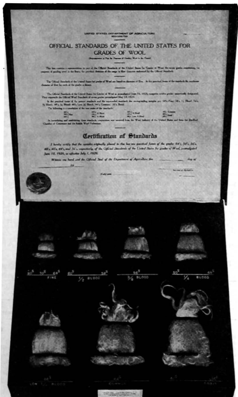
FIGURE 19.—CERTIFIED SAMPLES OF WOOL DISTRIBUTED BY THE U. S. DEPARTMENT OF AGRICULTURE FOR USE IN GRADING.
