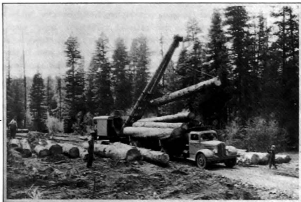
FIGURE 11.—TRUCK LOGGING IN THE PONDEROSA-PINE REGION Logs are being loaded for the haul to the railroad several miles away.
