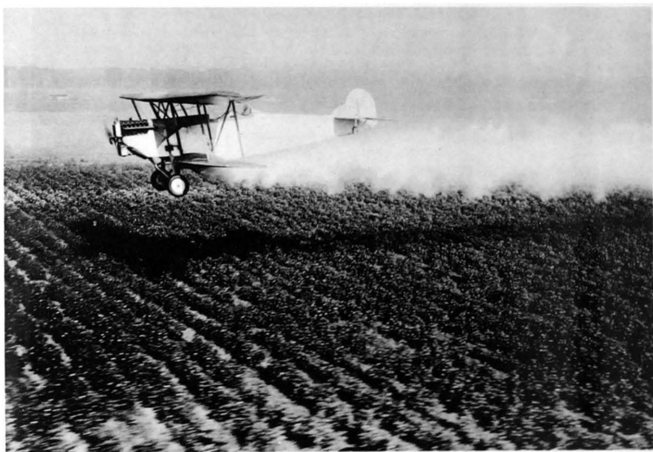
Aeroplane discharging calcium arsenate dust over cotton field for control of cotton boll weevil.
