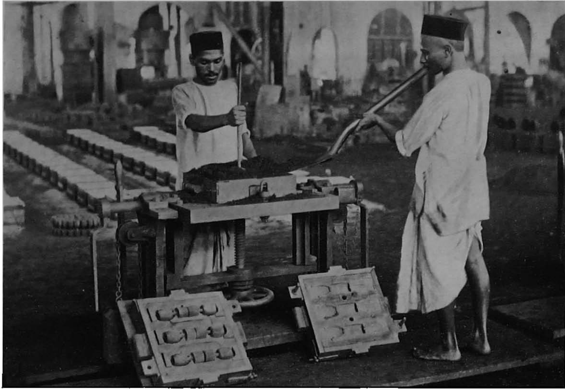
G.I.P. RAILWAY WORKS. MOULDING HAND GRENADES. (By kind permission of the Agent, G.I.P. Railway.)
