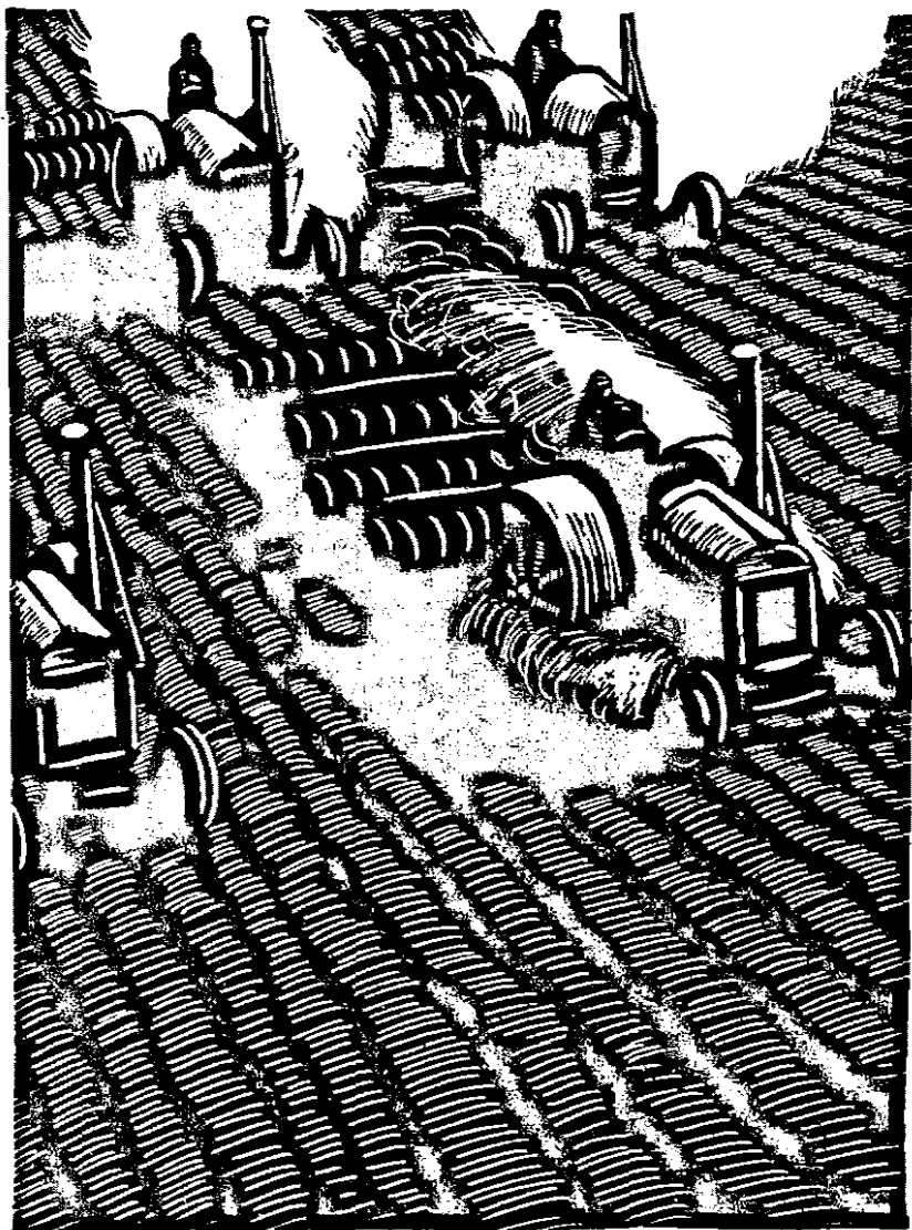
A DETACHMENT OF TRACTORS STARTS OUT TO WORK. EACH TRACTOR TOWS NOT ONE BUT SEVERAL HARROWS. THE HARROWS HAVE DISKS INSTEAD OF TEETH. THE DISKS HAVE SHARP EDGES
